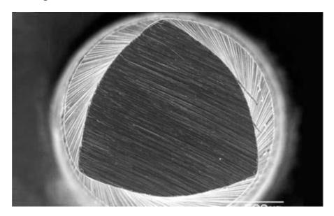
Its eccentric, it's not really centralized along the long axis of the file with rounded transition angles.
