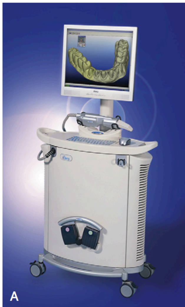
FIGURE 14.2 Digital impression systems. A , iTero. B , Lava Chairside Oral Scanner C.O.S. C , CEREC AC. (A, Courtesy of Cadent, Inc., Carlstadt, NJ; B, Courtesy of 3M ESPE, St. Paul, MN; C, Courtesy of Sirona, Charlotte, NC.)
