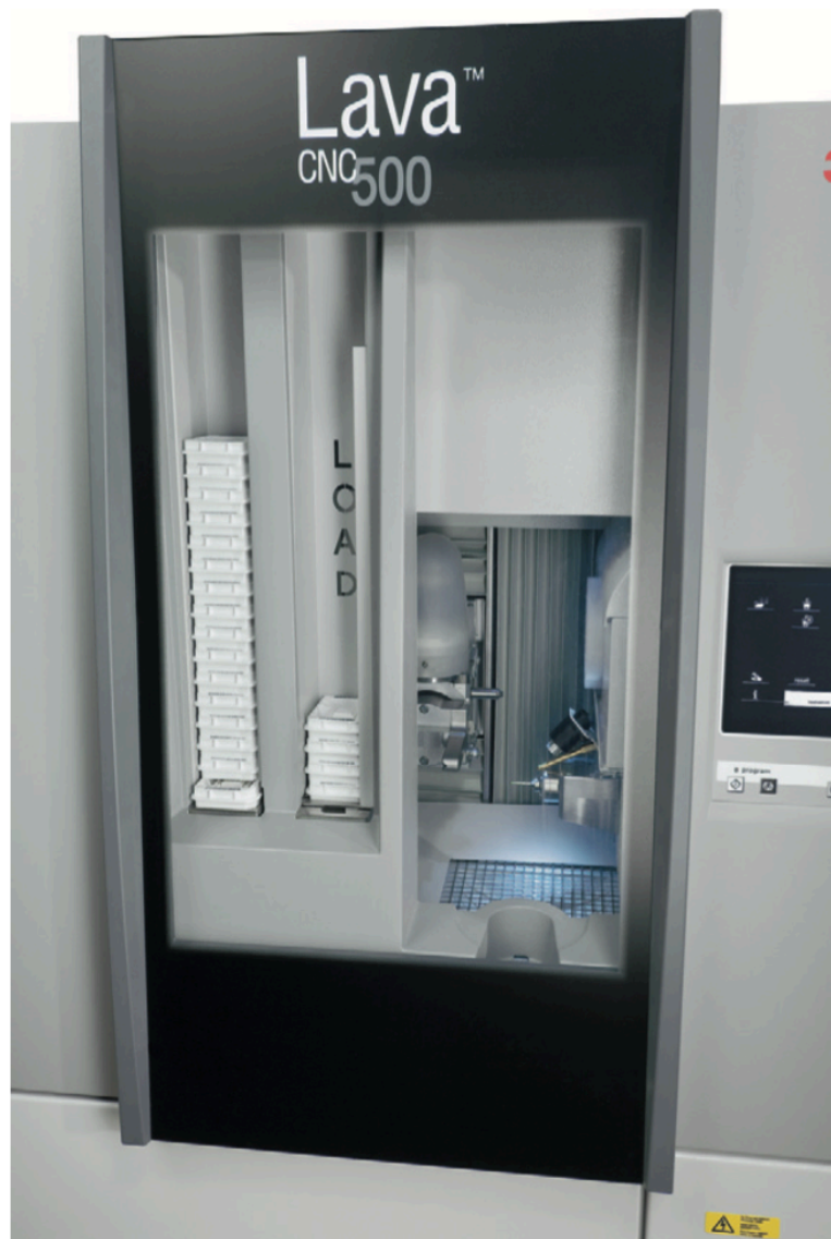
Figure 11.15 The Lava milling machine. The white rectangular zirconia blanks can be seen stacked up to the left, the millin machine is to the right.
