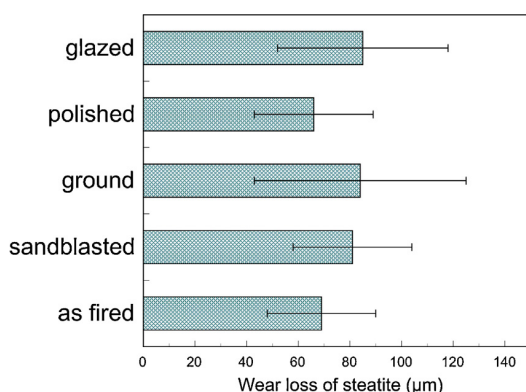
Fig. 18. Wear loss of steatite balls ( \phi = 6 mm) against five surface-treated zirconia after 5000 cycles. Graphing of the data in [113].
